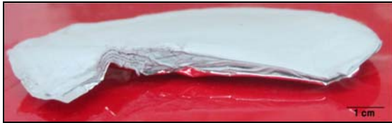
FIGURE 7. Compacted thick bulk structure of nanofibers deposited on solid substrate with high packing density.
