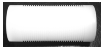
FIGURE 2. Solospun roller with thick teeth of 0.2 mm.
