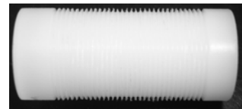
FIGURE 1. Solospun roller with thick teeth of 0.1mm.
