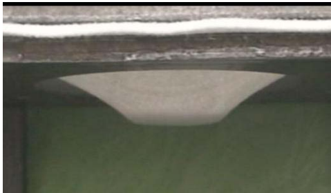
FIGURE 4. Deformation of geotextile layer during CBR test in A-B region.
