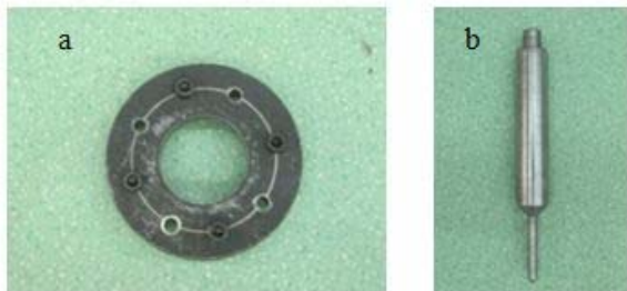
FIGURE 2. (a)Puncture test clamp. (b)Puncture test plunger.
