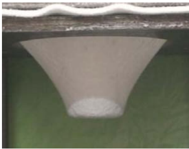
FIGURE 5. Deformation of geotextile layer during CBR test in A-B region.
