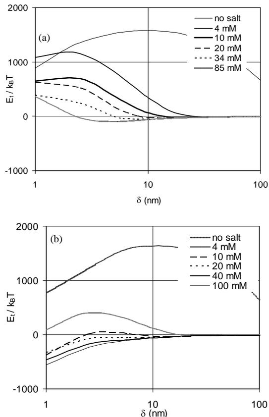
FIGURE 3. Calculated DLVO interaction energies for microsphere-fiber-water system as a function of separation distance: (a) in presence of Sodium chloride, (b) in presence of Calcium chloride.
