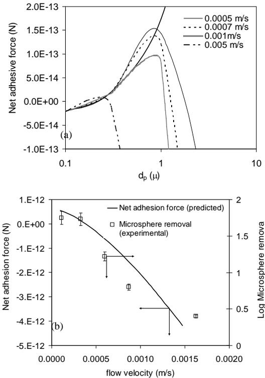
FIGURE 1. (a) Effect of flow velocity on net adhesion of particles on a cylindrical collector, (b) Effect of flow velocity on removal of  $3\ \mu\text{m}$  microspheres from a bed of fibrous media.
