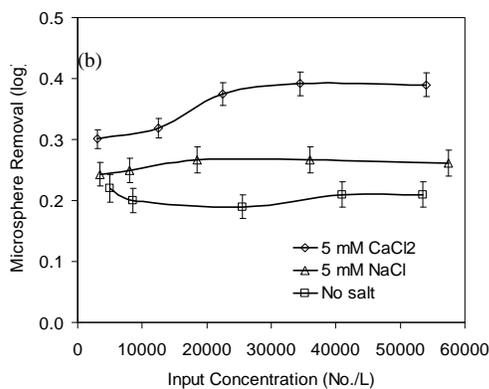
FIGURE 2. (a) Role of ionic strength on removal of microspheres from a bed of fibrous media, (b) Role of input concentration of the microspheres on removal in presence of sodium chloride and calcium chloride.
