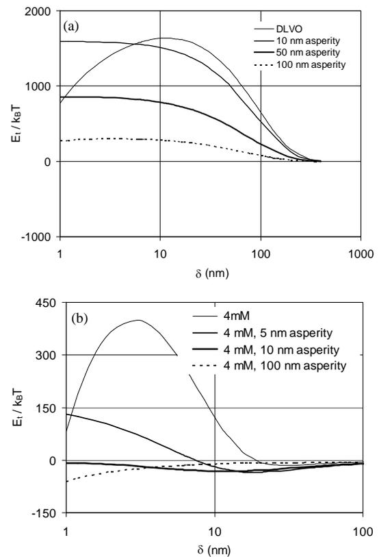
FIGURE 6. Calculated DLVO interaction energies for microsphere-fiber-water system as a function of separation distance due to surface roughness: (a) In absence of any added salt (b) in presence of 4 mM Calcium chloride.
