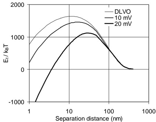
FIGURE 7. Predicted energy profiles for microsphere-fiber-water system in presence of charge heterogeneity of collector and microspheres without any added salt.
