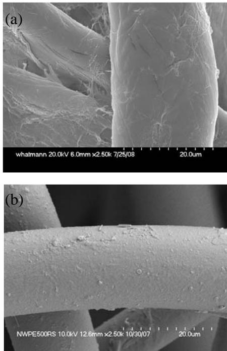
FIGURE 4. Scanning electron microscopy of (a) Whatman filter paper and (b) nonwoven polyester.
