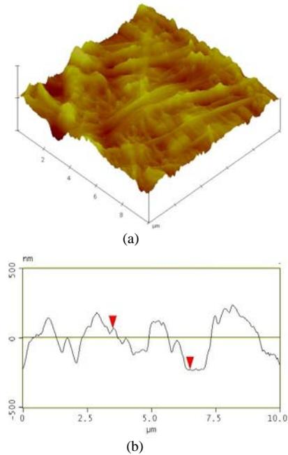
FIGURE 5. Surface roughness as measured by AFM technique for Whatman filter paper (a) 3D image, (b) 2D image
