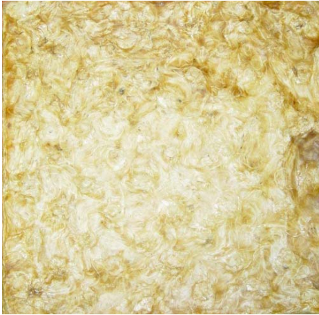
FIGURE 7. Insulating material board using Corn Starch resin (0.28 x 0.28 x 0.02113 m 3 ) with density of 265.63 kg/m 3 .
