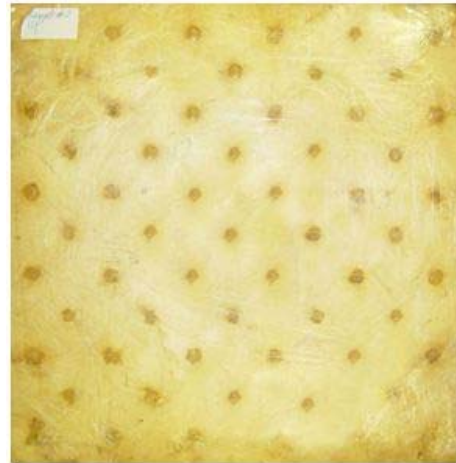
FIGURE 5. Insulating material board using the Phenol - Formaldehyde resin (0.3 x 0.3 x 0.0235 m)
