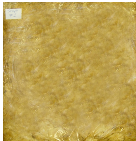
FIGURE 6. Insulating material board using the Phenol-Formaldehyde resin (0.283 x 0.283 x 0.02477 m).
