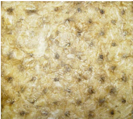
FIGURE 8. Insulating material board using cornstarch resin (0.30 x 0.29 x 0.020615 m 3 ) with density of 130.47 kg/m 3 .
