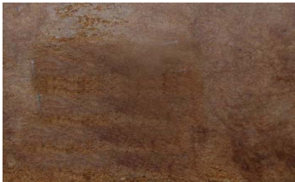
FIGURE 1. Jute reinforced polypropylene Composite Board
