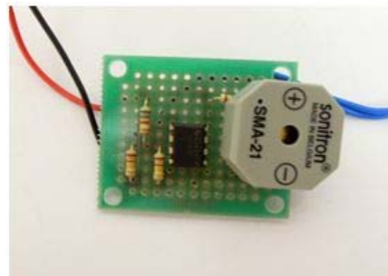
FIGURE 6. The developed prototype of siren signal system.
