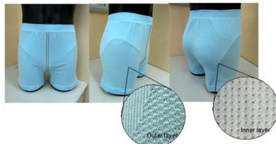
FIGURE 3. The developed prototype of incontinence monitoring pant in different views.
