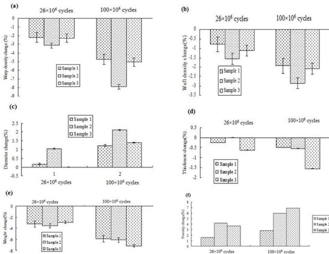
FIGURE 2. Properties of woven tubular samples after fatigue testing: (a) Warp density, (b) Weft density, (c) Filament diameter, (d) Thickness, (e) Mass per unit area, (f) Porosity.
