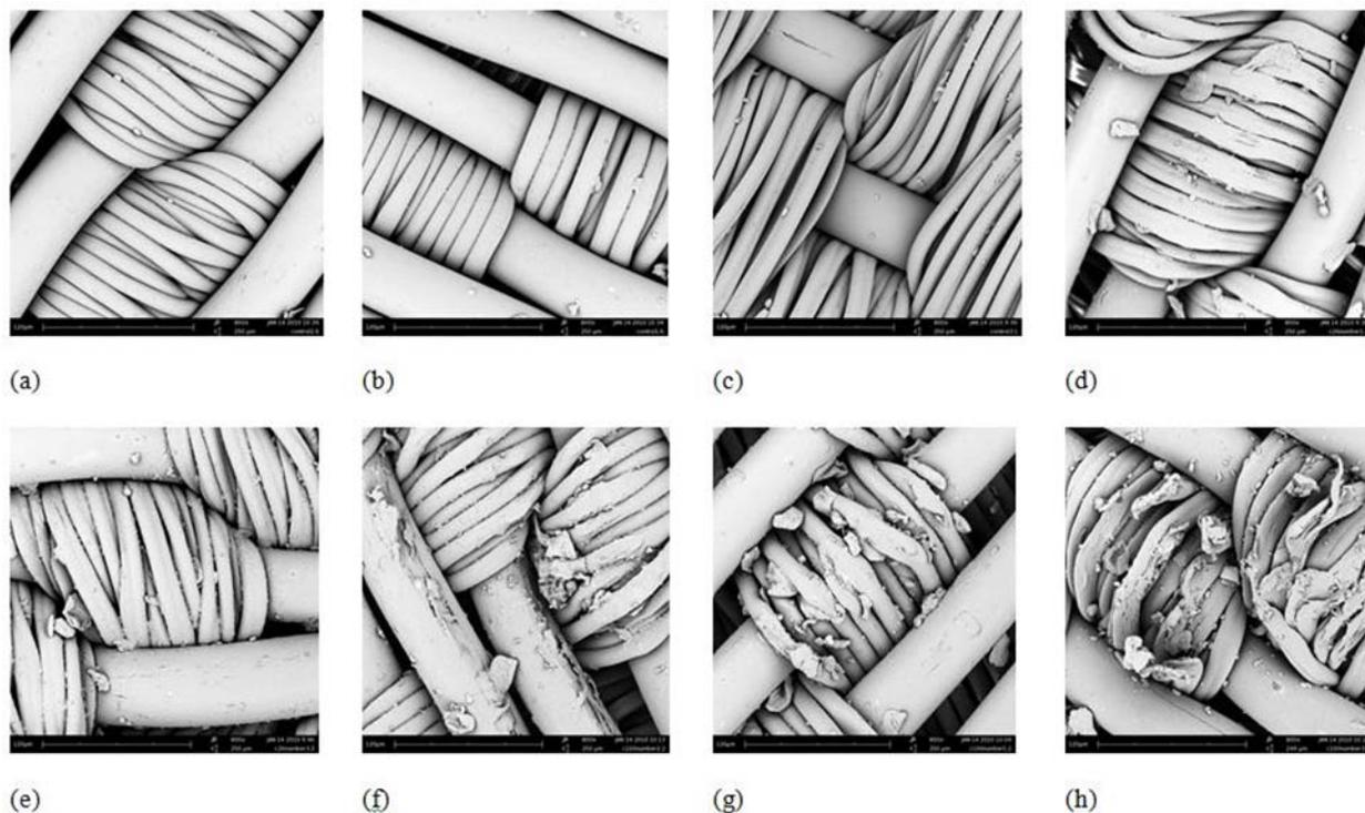
FIGURE 3. SEM photomicrograph of samples' internal surface (Magnification 800×): (a) Control sample 1; (b) Control sample 2; (c) Control sample 3; (d) Sample 2 after  $26 \times 10^6$  fatigue cycles; (e) Sample 3 after  $26 \times 10^6$  fatigue cycles; (f) Sample 1 after  $100 \times 10^6$  fatigue cycles; (g) Sample 2 after  $100 \times 10^6$  fatigue cycles; (h) Sample 3 after  $100 \times 10^6$  fatigue cycles.
