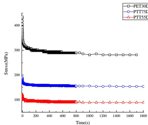
FIGURE 1. The stress relaxation curve of yarn samples at 10 % elongation rate.
