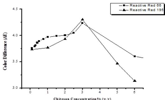
FIGURE 5. Relationship between chitosan concentration and color difference of dyed silk yarns treated with different amounts of chitosan on silk yarns dyed with reactive red 66 and reactive red 195.
