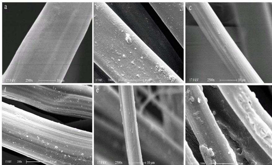
FIGURE 2. SEM photographs of the surface of silk yarns. (a) Untreated and undyed silk yarns (b) 3% chitosan treated undyed silk yarns (c) Untreated dyed silk yarns with reactive Red 66 (d) 3% chitosan treated dyed silk yarns with reactive Red 66 (e) Untreated dyed silk yarns with reactive Red 195 (f) 3% chitosan treated dyed silk yarns with reactive Red 195.
