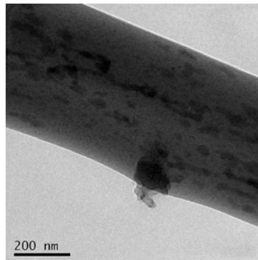
FIGURE 6. TEM images of PVAc/TiO<sub>2</sub> nanofibers.
