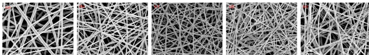
FIGURE 1. SEM images of the electrospun PVAc nanofiber membranes with different  $\text{TiO}_2$  contents (a) 0 wt%, (b) 0.25 wt% (c) 0.5 wt% (d) 0.75wt% (e) 1wt%.
