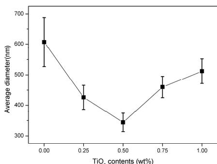
FIGURE 2. Average diameters of PVAc/TiO<sub>2</sub> nanofiber membranes with different TiO<sub>2</sub> contents.
