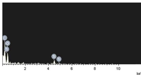
FIGURE 7. EDX spectra of PVAc/TiO<sub>2</sub> nanofibers.
