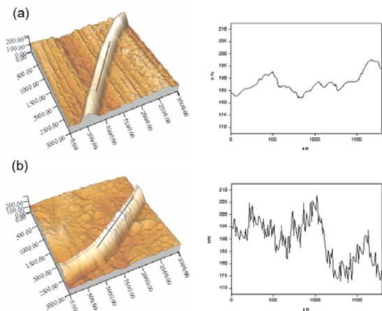
FIGURE 5. AFM images and the cross section profiles along the marked directions (a) PVAc and (b) PVAc/TiO<sub>2</sub> nanofiber.
