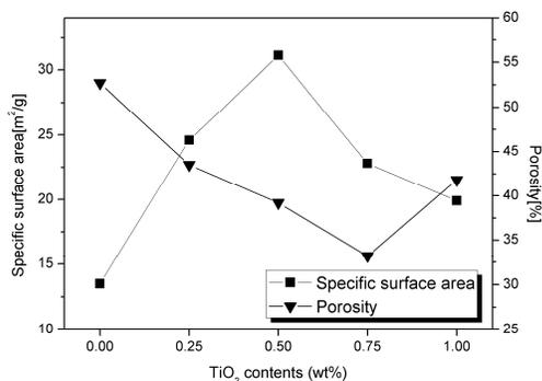
FIGURE 3. Specific surface area and porosity of PVAc/TiO<sub>2</sub> nanofiber membranes with different TiO<sub>2</sub> contents.
