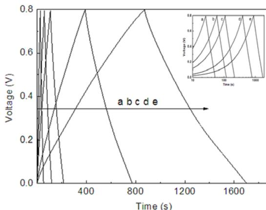
FIGURE 4. Charge-discharge behavior at different current densities (A/g). (a) 0.5, (b) 2.5, (c) 5.0, (d) 15.0, (e) 25.0.
