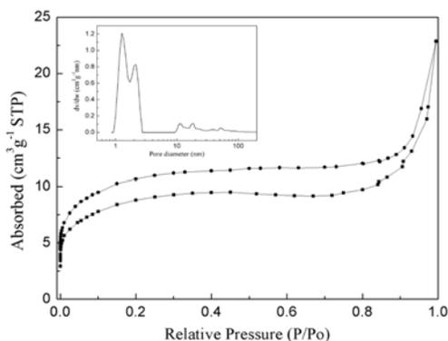
FIGURE 3. Nitrogen adsorption-desorption isotherms and pore size distribution curves of C/Ni composite nanofibers.
