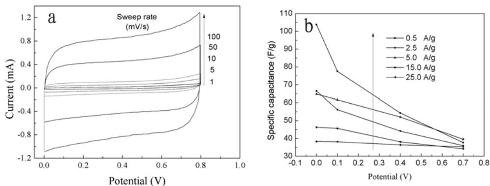
FIGURE 5. CVs of composite electrodes at different scan rate (a) and the specific capacitance as a function of voltage at different current densities (b).
