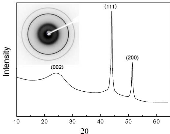
FIGURE 1. XRD pattern of the C/Ni composite nanofibers annealed at 800 °C. Inset: 2D X-ray image for the same sample.
