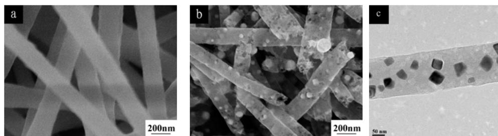
FIGURE 2. SEM images (mag.: ×50k) of PAN/PVP/Ni(OAc)<sub>2</sub> precursor (a), carbonized composite nanofibers (b), and TEM image of carbonized composite nanofibers (c).
