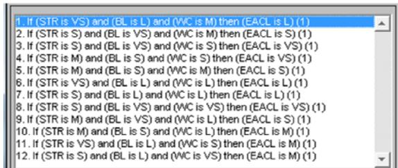
FIGURE 7. Fuzzy rules for ease allowance at crotch length (EACL).
