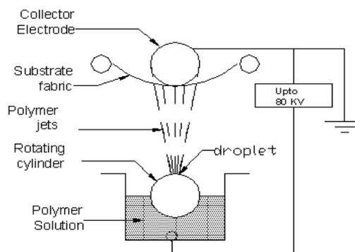
FIGURE 1. Schematic diagram of nano spider.
