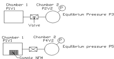
FIGURE 4. Schematic diagram of Pycnometer without and with sample.
