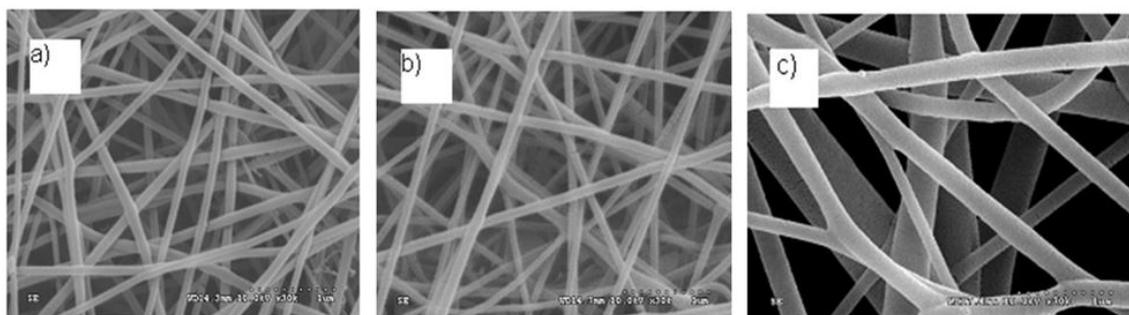
FIGURE 3. Microstructure of nano fiber of a) 0.6 GSM, b) 0.4 GSM, c) 0.23 GSM.
