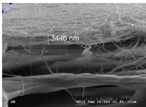
FIGURE 5. SEM images of the cross section of the nanofiber mats of 0.6 GSM on filter medium indicating its thickness.
