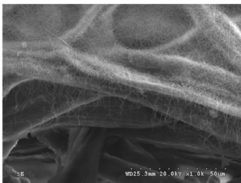
FIGURE 2. Nano fiber coated on the filtration medium.
