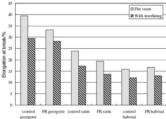
FIGURE 2. Breaking elongation of silk fabrics (FR means flame retardant treated).
