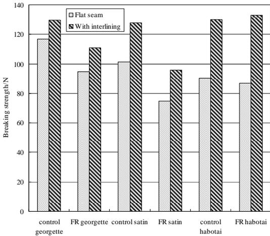
FIGURE 1. Breaking strength of silk fabrics (FR means flame retardant treated).
