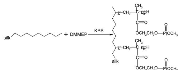
Scheme 2. Graft polymerization of silk with DMMEP.
