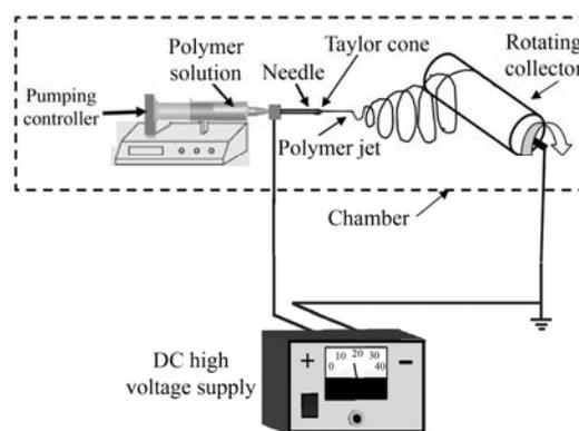
FIGURE 1. Schematic of electrospinning apparatus.
