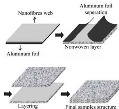
FIGURE 2. Schematic of prepared sample.
