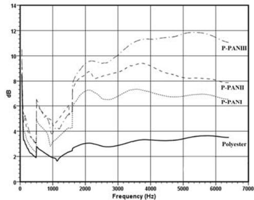
FIGURE 5. Changes of sound transmission loss against frequency; different number of PAN nanofiber layers within polyester layers.
