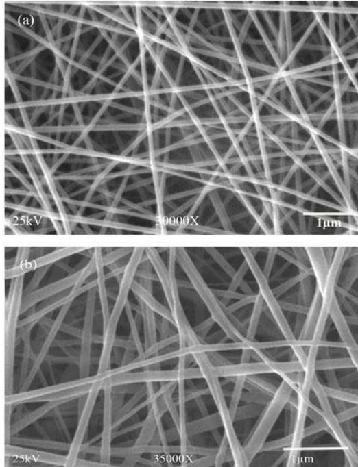
FIGURE 3. SEM micrograph of surface morphology of (a): PAN and (b): PU nanofibers.
