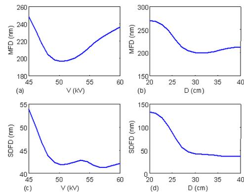
FIGURE 5. (a): Impact of applied voltage on MFD while spinning distance is held constant (D= 30 cm); (b): Impact of spinning distance on MFD while applied voltage is held constant (V=50 kV); (c) Impact of applied voltage on SDFD while spinning distance is held constant (D=30 cm); and (d): Impact of spinning distance on SDFD while applied voltage is held constant at (V=50 kV).
