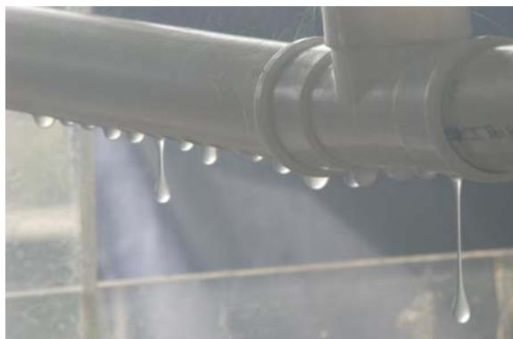
FIGURE 2. Image of solution distributor.
