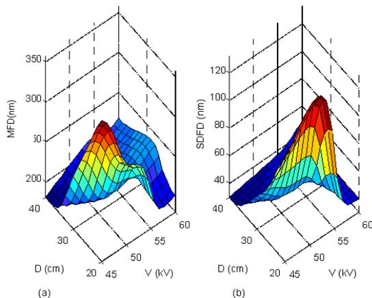
FIGURE 6. Combined effects of electrospinning distance and applied voltage on (a): MFD; (b) SDFD.
