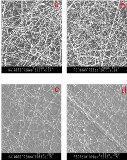
FIGURE 3. SEM (X2000) images by splashing needleless method (a): V=45kV; d=25cm; (b): V=50kV; d=20cm; (c) V=50kV; d=40cm; (d) V=50kV; d=30cm.
