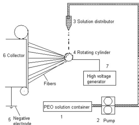
FIGURE 1. Splashing electrospinning setup.
