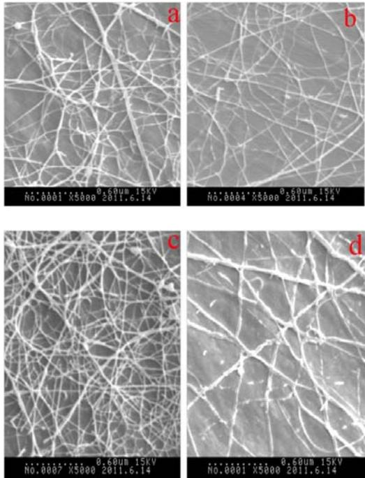
FIGURE 4. SEM (X5000) images by splashing needleless method (a): V=60kV; d=35cm; (b): V=60kV; d=20cm; (c): V=60kV; d=30cm; (d): V=45kV; d=20cm.
