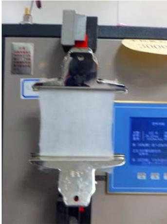
FIGURE 2. Equipment for the cohesive force measurement.
