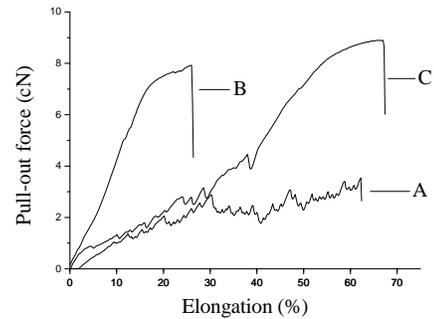
FIGURE 3. Pull-out curves of fibers from the spunlaced nonwoven fabric.
