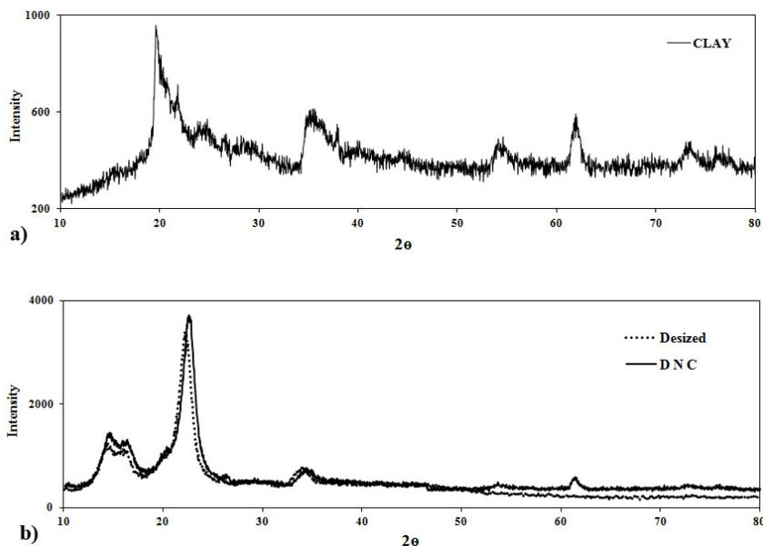
FIGURE 5. XRD patterns of clay (a) and selected denim garments (b).
