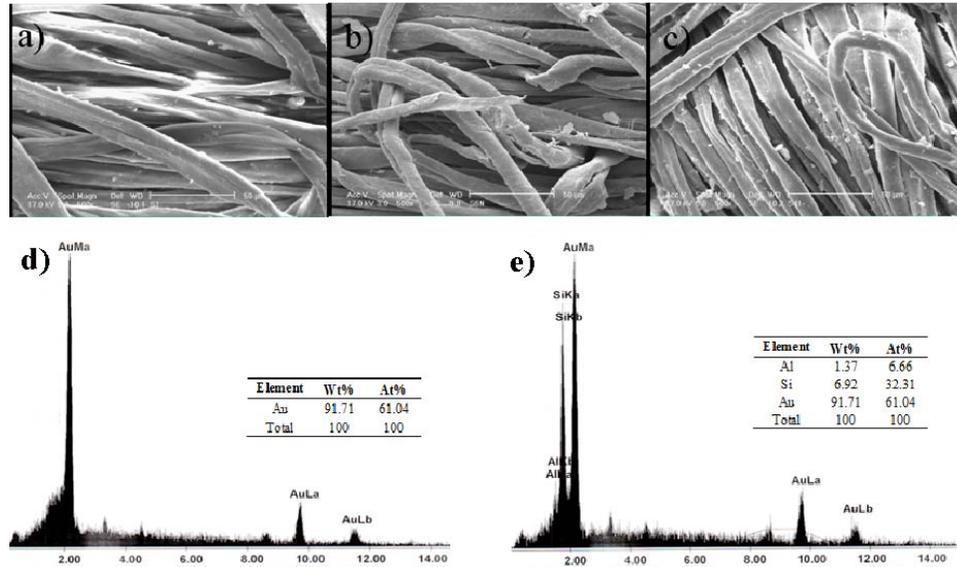
FIGURE 2. SEM images of different treated denim garments (500 $\times$ ); desized (a), treated with cellulases (b), treated with clay (c), EDAX of desized or treated with cellulase (d) and treated with nanoclay (e).
