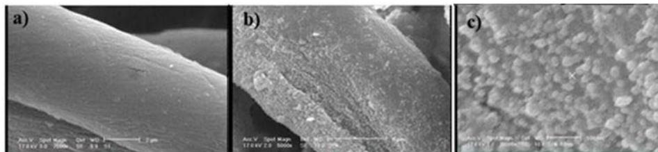
FIGURE 3. SEM images of different treated denim garments with cellulases (a), nano clay (b), and morphology of nano clay on surface of treated fiber (c).
