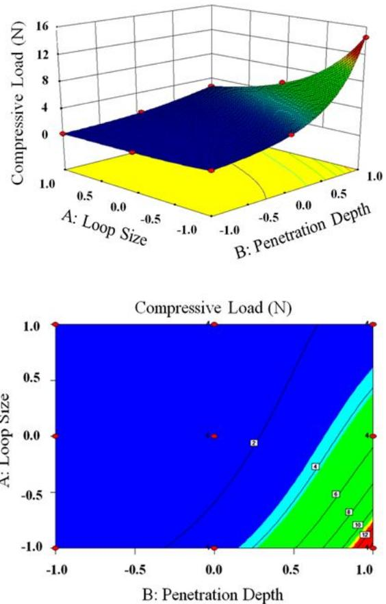
FIGURE 5. Effects of loop size and penetration depth on the compressive load (three dimensional and layer graphs).
