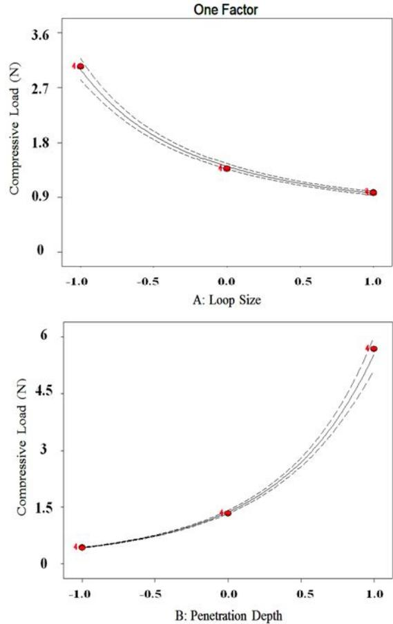
FIGURE 3. Effects of loop size and penetration depth on the compressive load (A: loop size, B: penetration depth).
