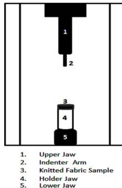
FIGURE 1. Experimental set up for measuring the compressive force by Instron Tensile Tester.
