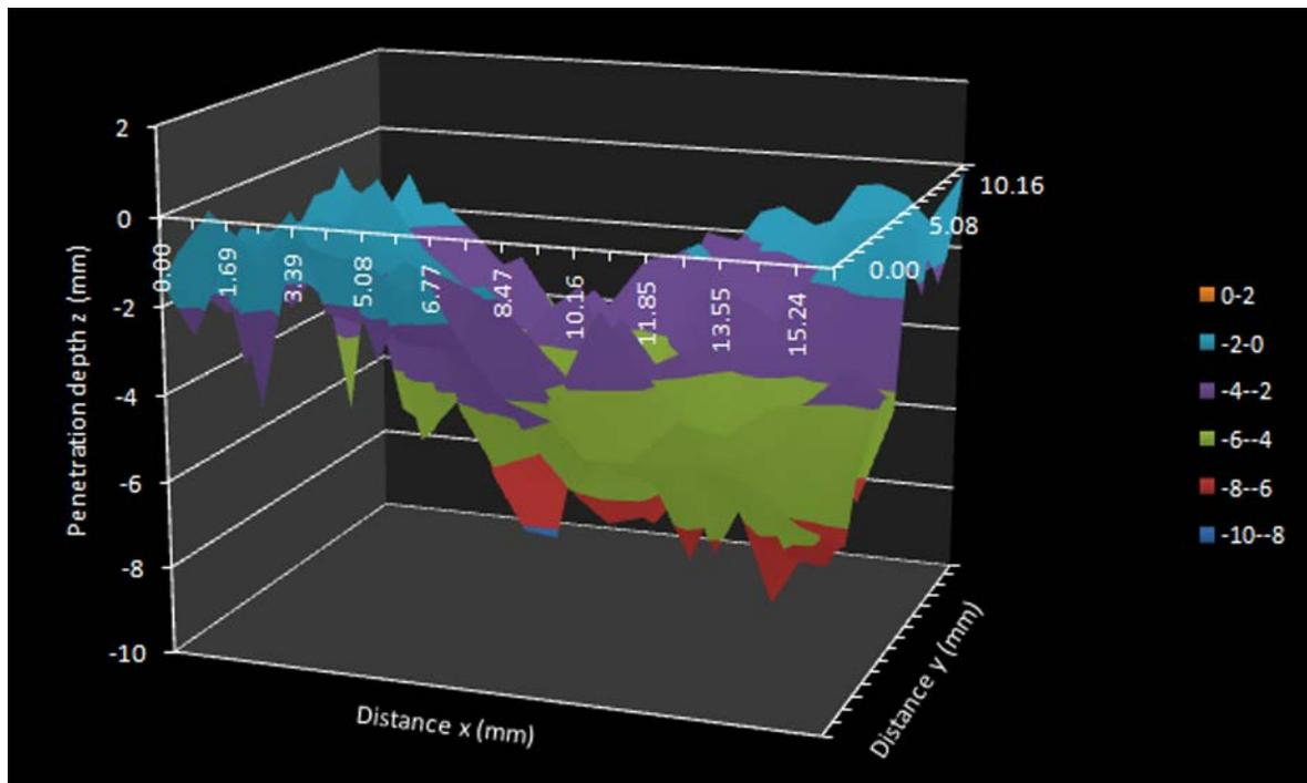
FIGURE 8. Penetration depth analysis of shot No.1
