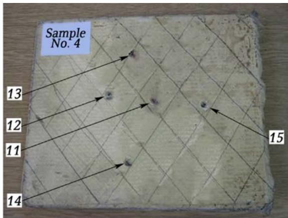
FIGURE 4. Front side of shot sample No.4.
