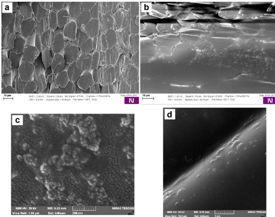
FIGURE 1. SEM image of : a) the *p*-aramid/PVB fabric composite (scale bar 10 μm); b) the *p*-aramid/PVB fabric composite with the 30 wt.% AMEO silane modified silica nanoparticles (scale bar 10 μm); c) the modified silica nanoparticles on the aramid fabric (scale bar 200 nm); d) the modified silica nanoparticles that entered aramid fibers of the fabric (scale bar 2 μm).
