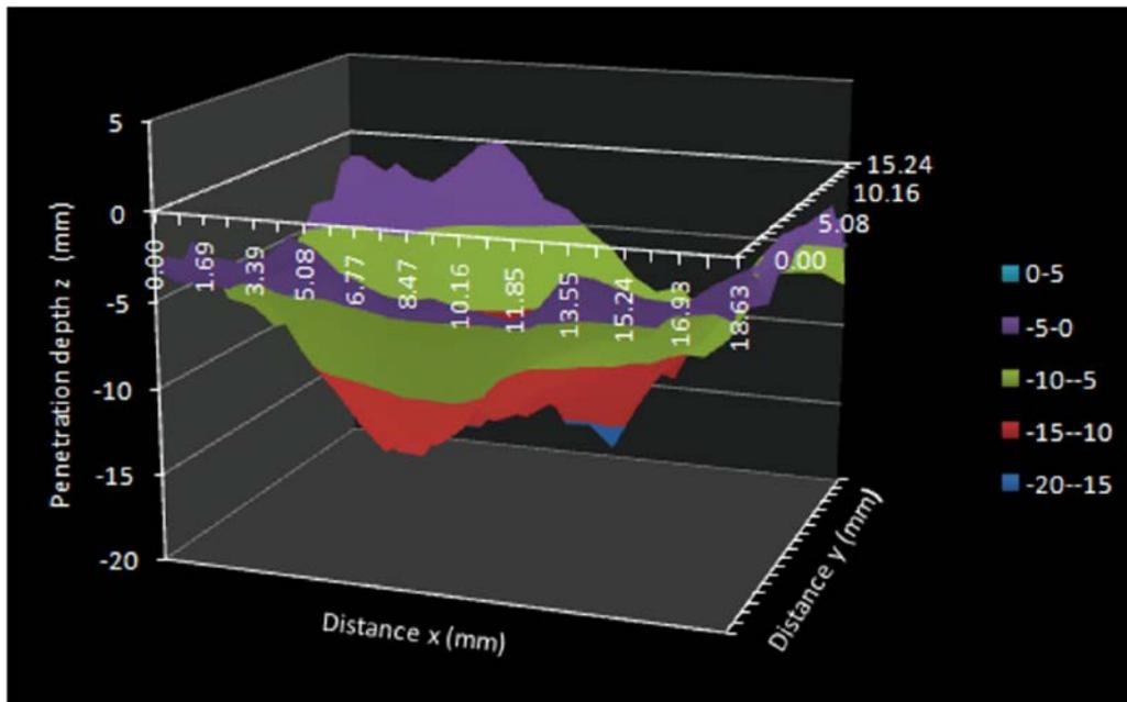
FIGURE 12. Penetration depth analysis of shot No.15.
