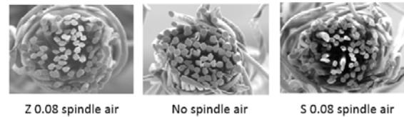
FIGURE 7. Structure of vortex yarn with different spindle air pressure.
