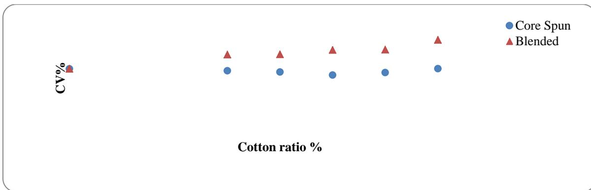
FIGURE 4. Evenness of core spun yarn and blended yarn at different PSA/cotton ratios.
