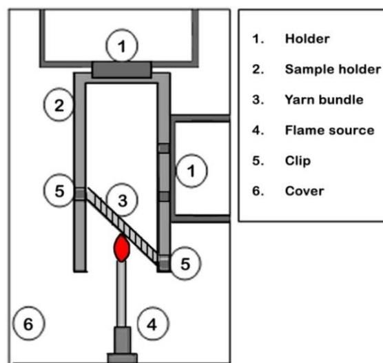
FIGURE 1. Schematic diagram of improvised flame retardant yarn tester.
