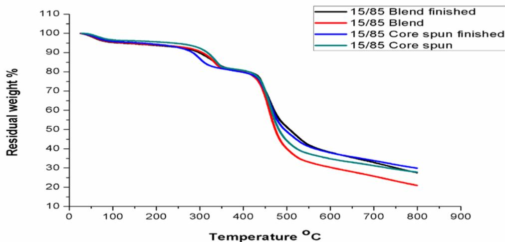
FIGURE 7. Themogravimetic analysis of 15/85 PSA/cotton ratio of finished corespun and blended yarns.
