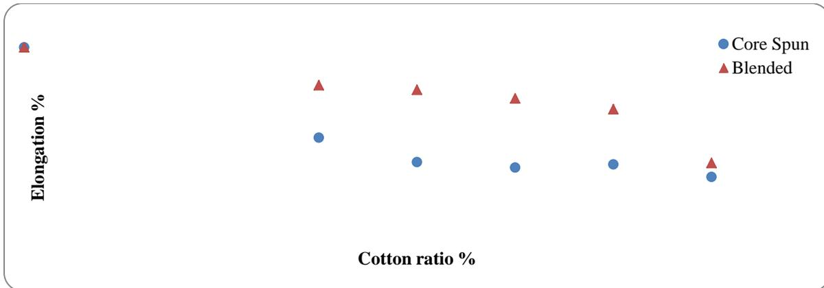
FIGURE 3. Elongation at break of core spun yarn and blended yarn at different PSA/cotton ratios.
