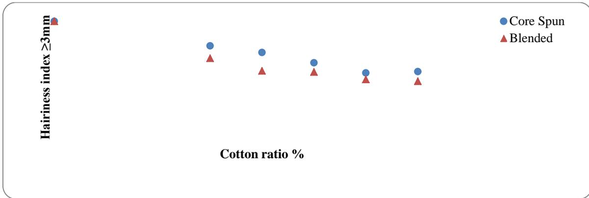
FIGURE 5. Hairiness of core spun yarn and blended yarn at different PSA/cotton ratios.
