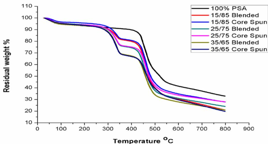
FIGURE 6. Themogravimetic analysis of different ratios of unfinished corespun and blended yarns.
