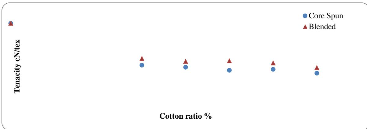
FIGURE 2. Tenacity of core spun yarn and blended yarn at different PSA/cotton ratios.
