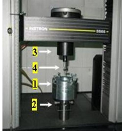
FIGURE 1. Experimental set up to measure needle penetration force on Instron tensile tester.
