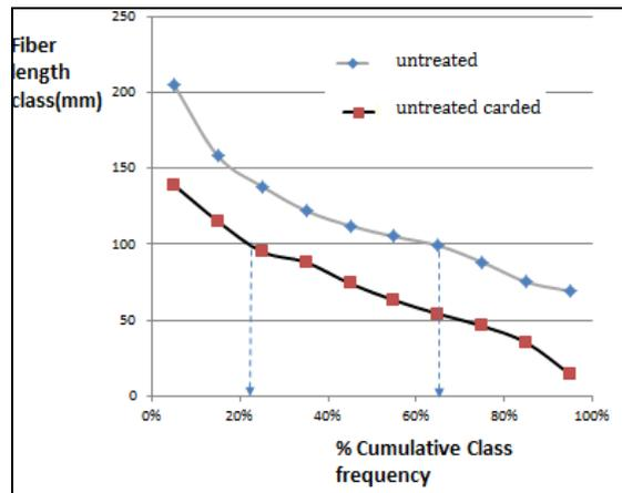
FIGURE 4. Cumulative frequency (%) plotted against fiber length class for the untreated flax fibers before carding (grey curve) and after carding (black curve).
