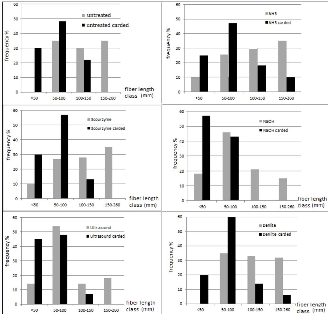
FIGURE 5. Frequency distribution of 4 different fiber length classes for the 5 different treatments, before carding (grey bars) and after carding (black bars).
