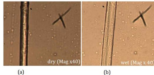
FIGURE 1. Microscopic views of a single flax fiber before (a) and after immersion in water for 1 hour (b)
