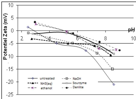
FIGURE 8. Zeta potential (mV) as a function of pH values for flax fibers with 5 pre-treatments.
