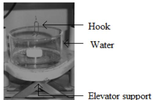
FIGURE 2. Wettability set-up, floating test.
