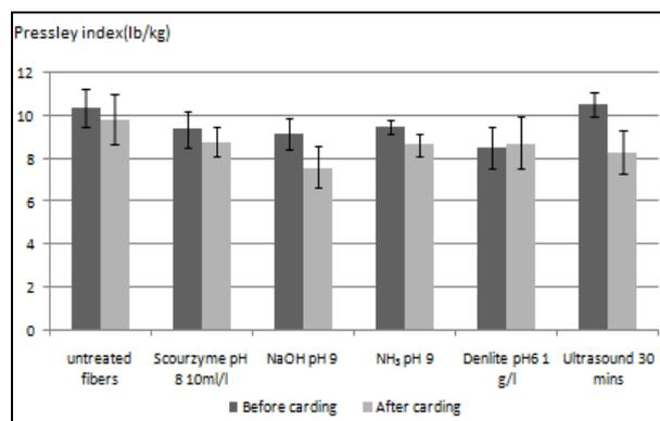
FIGURE 7. Flax fiber bundle tenacity for different pre-treatments before and after carding. The standard deviation values are presented by bar errors.
