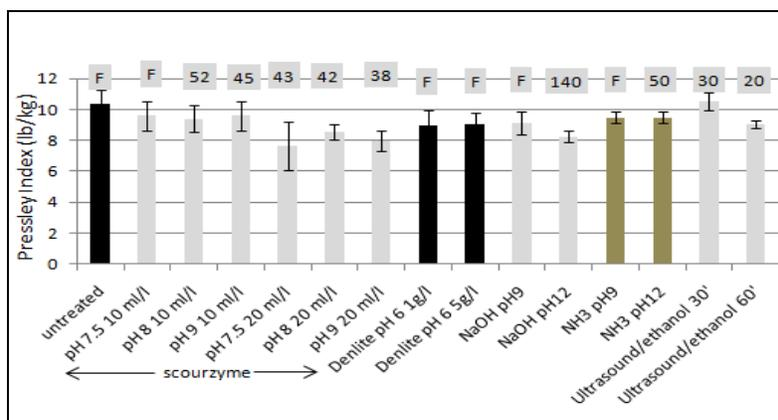
FIGURE 3. Tenacity (lb/kg) of flax fiber bundles. The wettability of fibers characterised using the floating test is expressed in terms of time taken in seconds for a floating horizontal fiber to fall down (to sink) when placed at the top of distilled water surface. 'F' in a grey square denotes that the fiber always floated.
