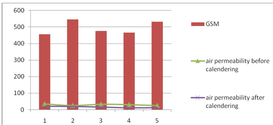
FIGURE 3. Relationship between GSM and air permeability.
