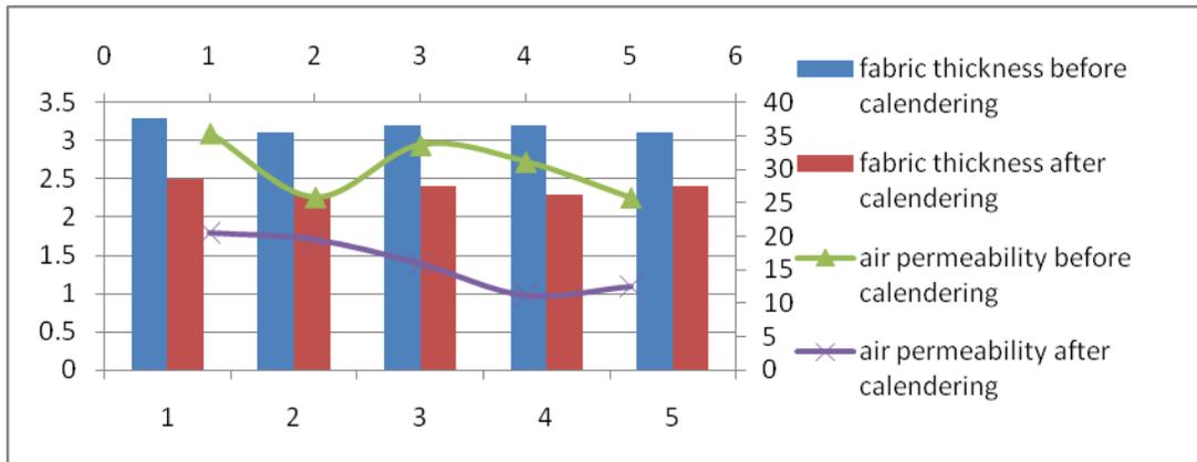
FIGURE 1. Relationship between fabric thickness and air permeability.
