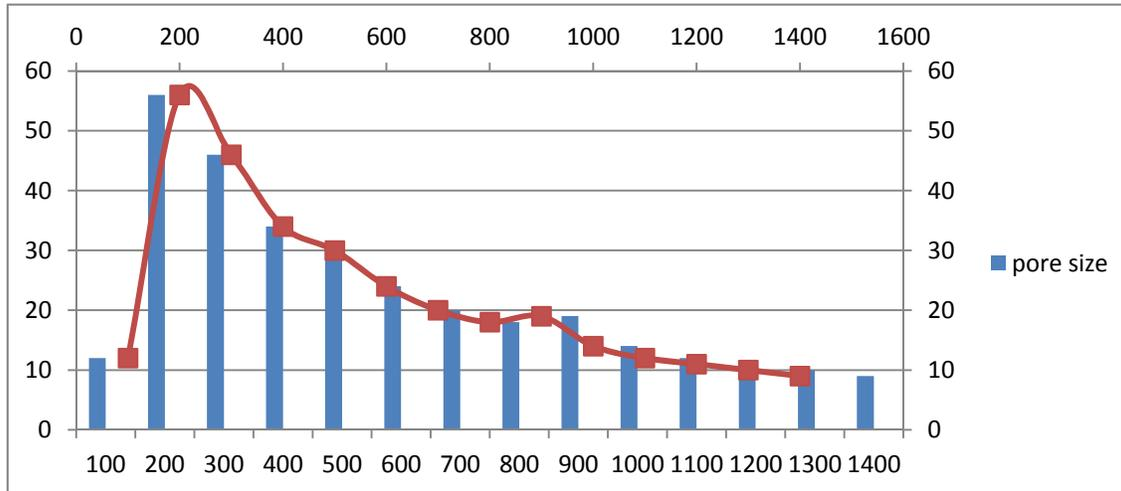
FIGURE 4. Sample 1 pore size and its distribution.
