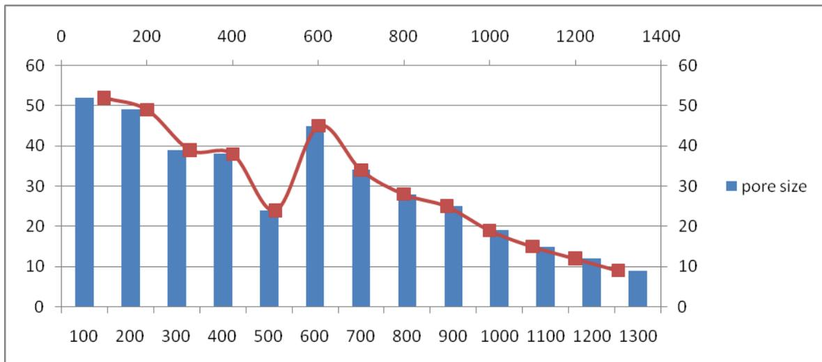
FIGURE 5. Sample 2 pore size and its distribution.
