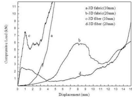
FIGURE 6. Load-displacement curves of flat compression tests on 3D fabric and 3D fiber composites.
