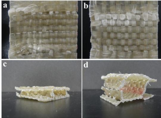
FIGURE 7 Breakage photographs of 3D fabric composites suffering flat compressive loads for face-sheet with core height of (a) 10mm and (b) 20mm and for core with core height of (c) 10mm and (d) 20mm.
