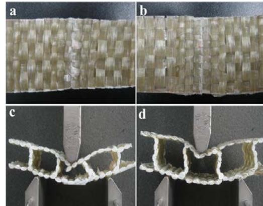
FIGURE 10. Breakage photographs of 3D fabric composites suffering flexural loads for face-sheet with core height of (a) 10mm and (b) 20mm and for core with core height of (c) 10mm and (d) 20mm.
