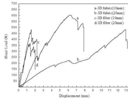
FIGURE 8. Load-displacement curves of shear tests on 3D fabric and 3D fiber composites.
