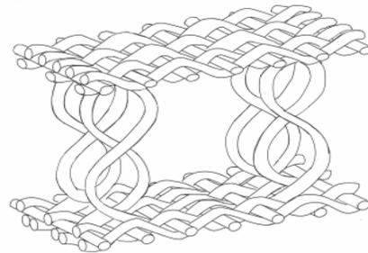
FIGURE 1. Schematic diagram of 3D fiber composites.
