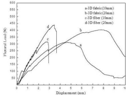
FIGURE 9 Load-displacement curves of flexure tests on 3D fabric and 3D fiber composites.
