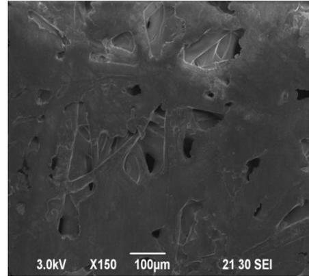
FIGURE 5. SEM Images of wool-fiber reinforced polypropylene composites.
