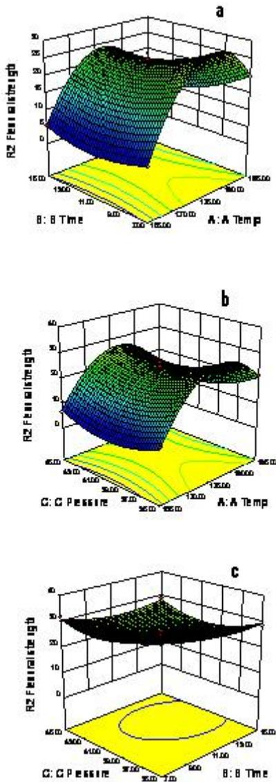
FIGURE 3. (a) Plot of effect of time and temperature on flexural strength (b) Plot of effect of pressure and temperature on flexural strength (c) Plot of effect of pressure and time on flexural strength.
