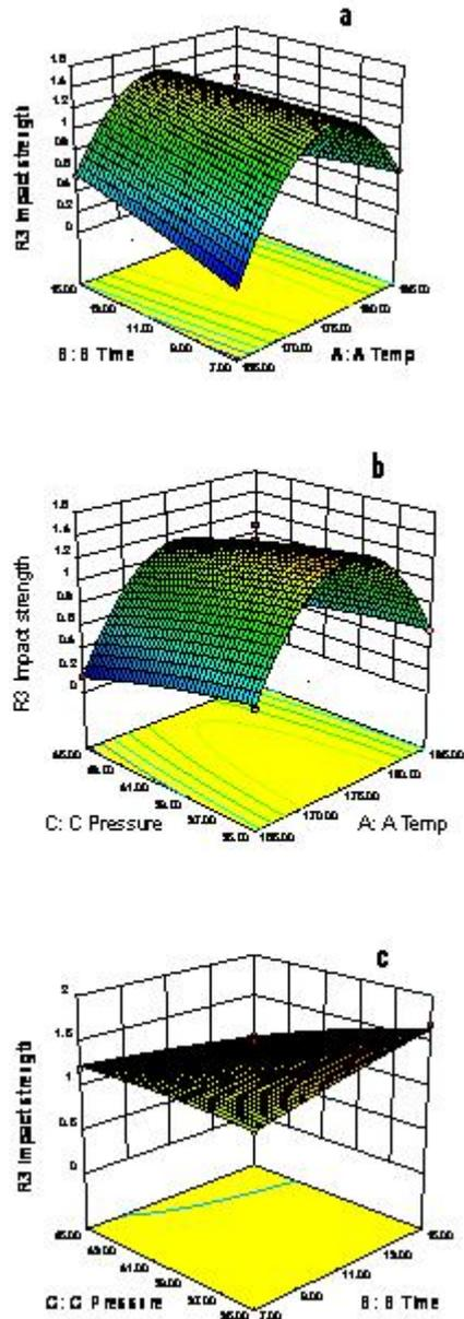
FIGURE 4. (a) Plot of effect of time and temperature on impact strength (b) Plot of effect of pressure and temperature on impact strength (c) Plot of effect of pressure and time on impact strength.
