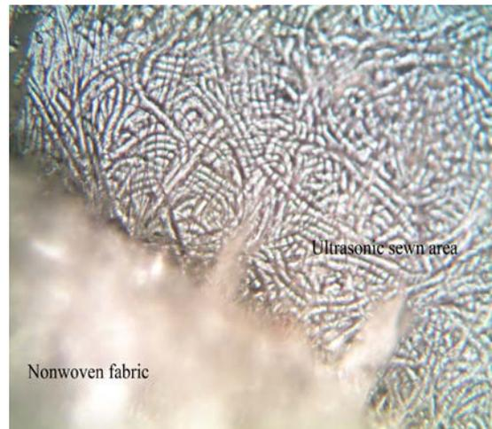
FIGURE 7. Microscopic images of ultrasonic seam area of the sewn nonwoven fabrics (x100).
