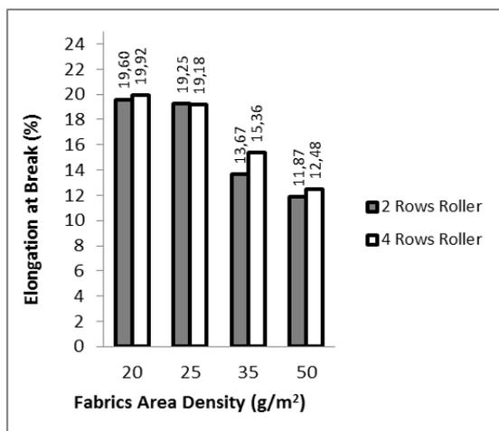
FIGURE 13. Elongation at break values of PA - PES fabric.
