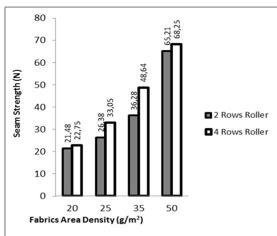
FIGURE 14. Ultrasonic seam strength values of PP fabric.
