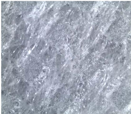
FIGURE 6. Microscopic image of the nonwoven fabric (x40).
