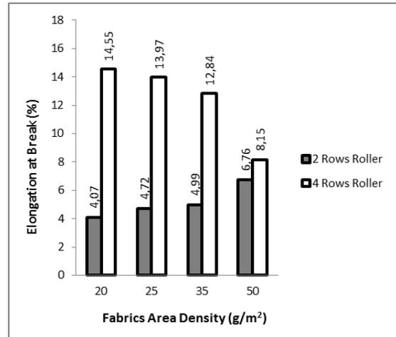
FIGURE 11. Elongation at break values of PES fabric.
