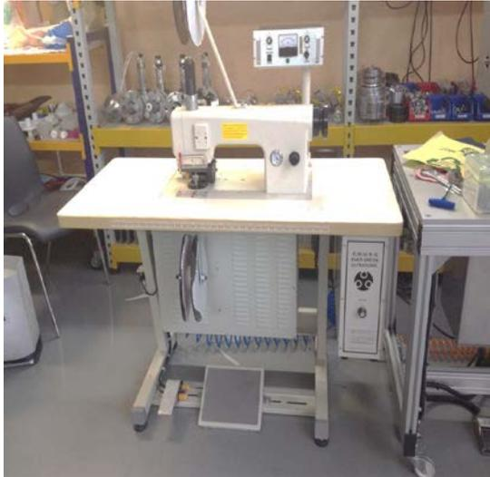
FIGURE 1. EGR – 015 Sonimak ultrasonic sewing machine.
