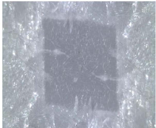
FIGURE 8. Microscopic images of the sewn nonwoven fabrics (x50).
