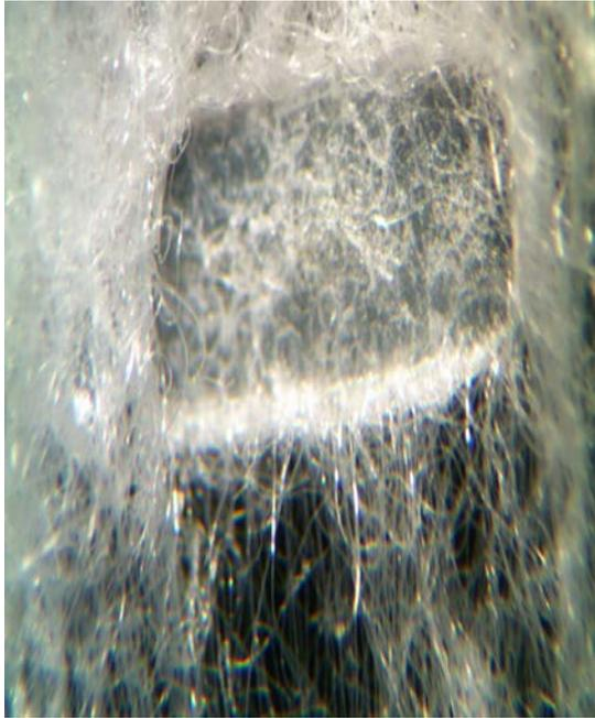
FIGURE 9. Microscopic images of the sewn nonwoven fabric after seam tensile test (x64).
