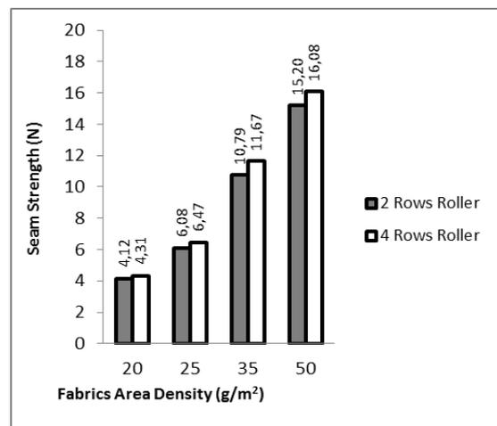
FIGURE 12. Ultrasonic seam strength values of PA - PES fabric
