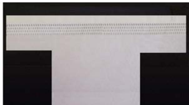
FIGURE 5. Photos of the sewn by 2 and 4 rows of roller nonwoven fabrics before seam strength test.
