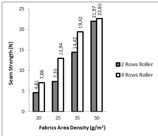
FIGURE 10. Ultrasonic seam strength values of PES fabric.
