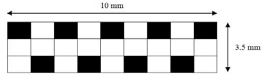
FIGURE 3. Sewing surface area for 2 rows roller.
