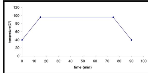
FIGURE 2. Time-temperature curve of sample dyeing.
