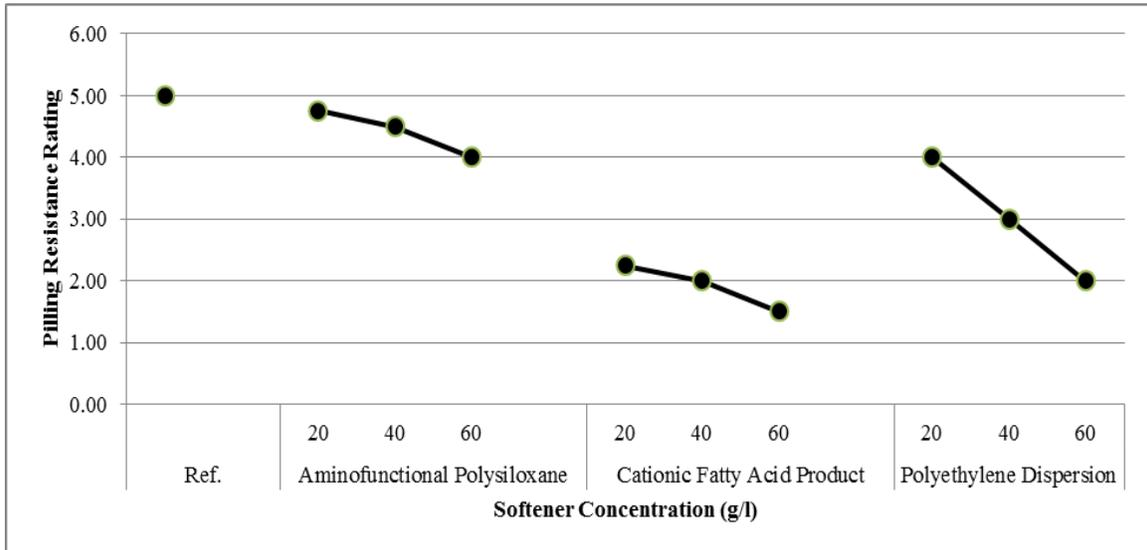
FIGURE 6. Effect of Different Softeners on Pilling Resistance of Knitted Fabrics.
