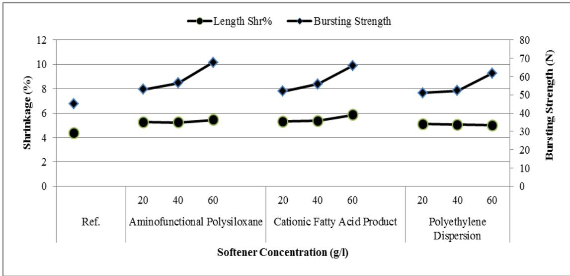
FIGURE 5. Effect of Different Softeners on Shrinkage and Bursting Strength of Knitted Fabrics.
