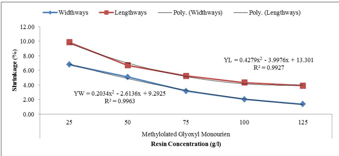
FIGURE 2. Effect of Methylolated Glyoxyl Monourien on shrinkage of knitted fabrics.
