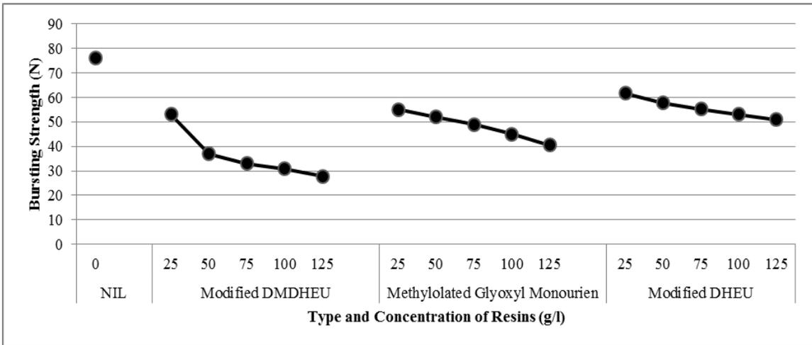
FIGURE 3. Effect of different resins on fabric bursting strength.
