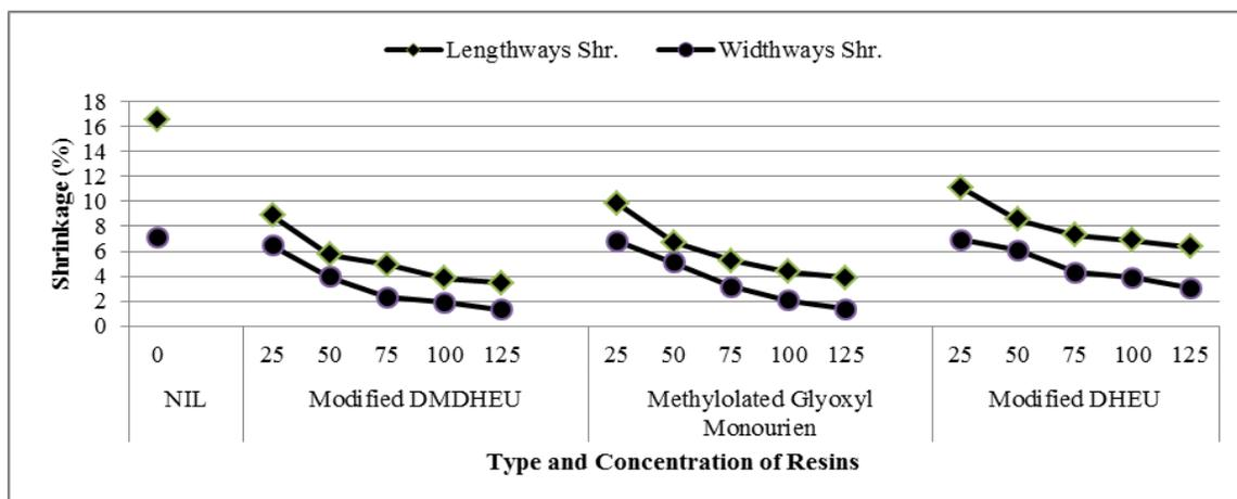
FIGURE 1. Effect of different resins on fabric shrinkage.
