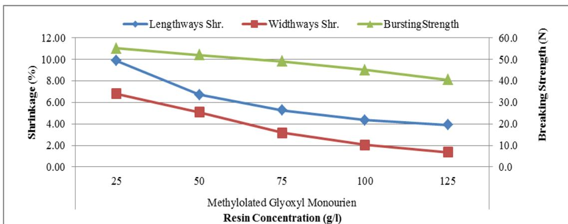
FIGURE 4. Effect of Methylolated Glyoxyl Monourien on shrinkage and bursting strength of knitted fabrics.
