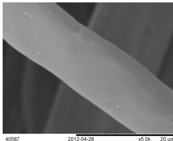
FIGURE 5. The morphology of scoured kapok fiber.
