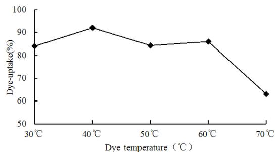
FIGURE 8. The relation between the dye-uptake on modified kapok fiber and the different dye temperature.
