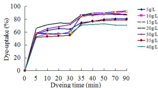
FIGURE 10. The relation between the dye-uptake on modified kapok fiber and the different concentration of fixing agent.
