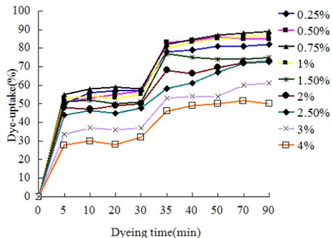
FIGURE 7. The relation between the dye-uptake on modified kapok fiber and the different concentration of reactive dye.
