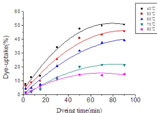
FIGURE 3. The relation between the dye-uptake on scoured kapok fiber and the different dye temperature.
