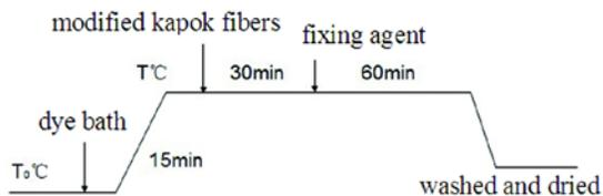
FIGURE 1. The dye process curve of reactive dyes.
