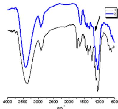
FIGURE 4. The infrared spectra of unmodified and modified kapok fiber, line 1 was unmodified kapok fiber, line 2 was modified kapok fiber.
