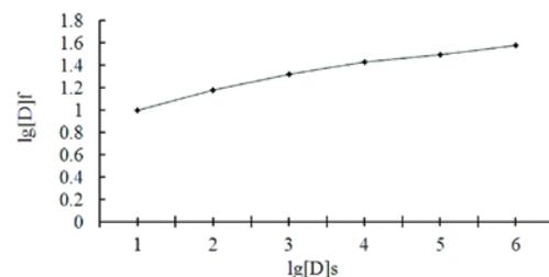
FIGURE 2. The relation between the  $\lg[D]_f$  and the  $\lg[D]_s$ ,  $[D]_f$  was the concentration of dye on the fiber and  $[D]_s$  was the concentration of dye in the dye bath.
