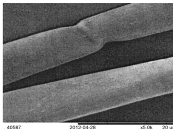
FIGURE 6. The morphology of cationic modified kapok fiber.
