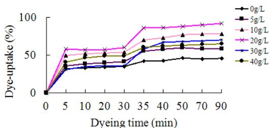
FIGURE 9. The relation between the dye-uptake on modified kapok fiber and the NaCl amount.
